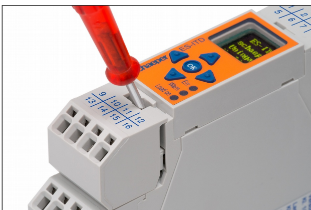
Figure 7.1: Removing plug-in terminals In device versions with plug-in terminals, these can be removed with the aid of a screwdriver.
